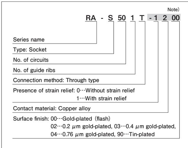
Note: The code -1200 is not shown for partially gold-plated flush with strain relief. For gold-plated flash products without strain relief, -0200 is indicated as -0.
