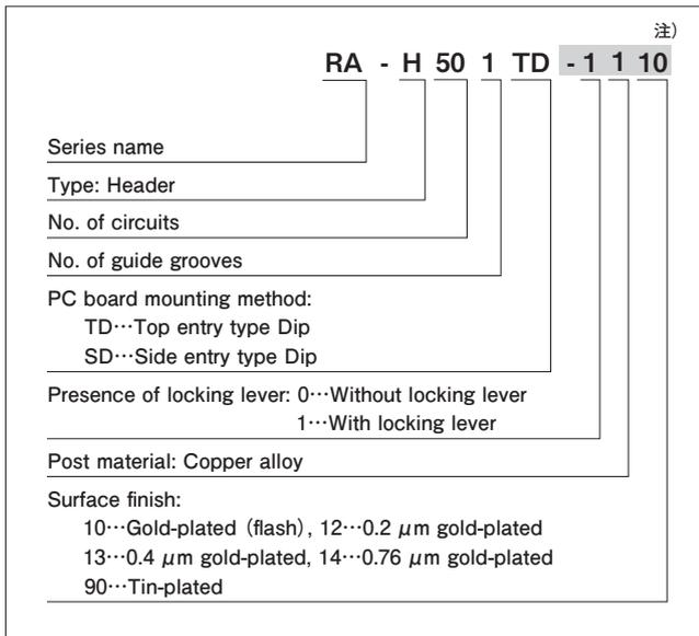
Note: The code -1100 is not shown for partially gold-plated flush products with lock levers.
